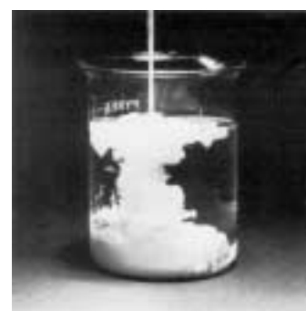
Fogging oil prepared with an Emulsifier added to water
