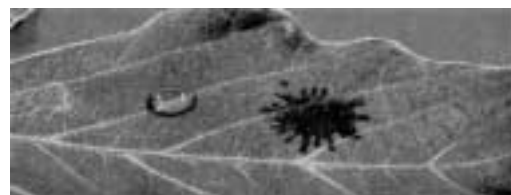
Efficacy of a wetting agent on the surface tension of a water droplet
