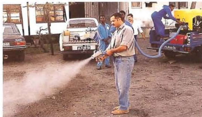
Conventional/High Volume Spraying Technique 100 - 500 Microns Droplet Size
