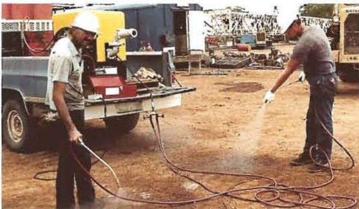
Larvaciding/Residual Spraying Technique 100 - 300 Microns Droplet Size
